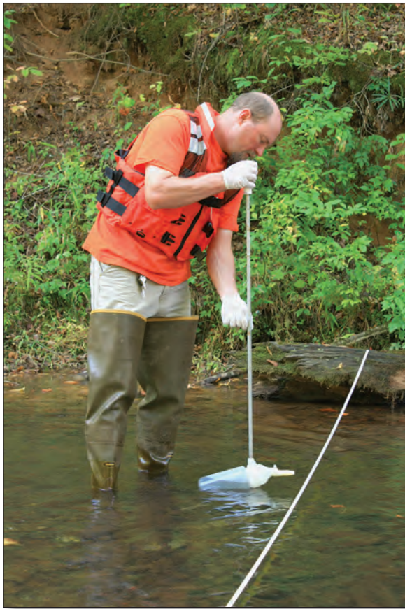
Figure 3–8. Water-quality samples were collected during base-flow conditions at sampling locations in each study area. These samples were analyzed for nutrients, dissolved pesticides and pesticide degradates, suspended sediment, sulfate, and chloride.
