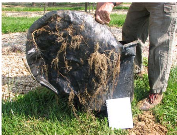
Figure 19. Ash roots penetrating geotextile after compacted subsoil has been washed away. Roots increased infiltration by a factor of 27. Photo by Susan Day.
