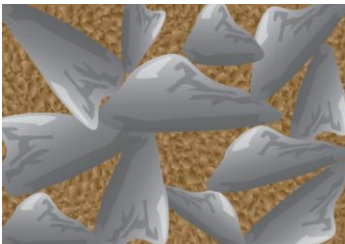
Conceptual diagram of structural soil (Bassuk, 2007)
