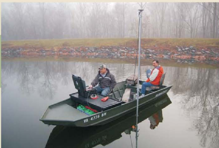
Bathymetric Survey using the EchoTrac System
